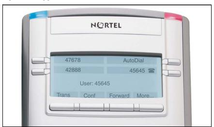
Figure 9: Logged in to an IP Phone 1120E
